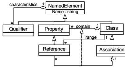
**Fig. 3.** CIM Metamodel (extracted from CIM Metaschema)
