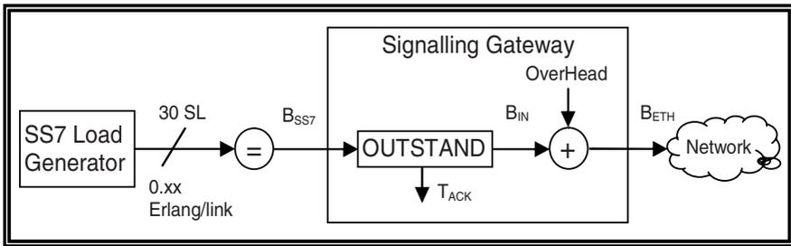
Fig. 10. System under Test transmitting scheme
