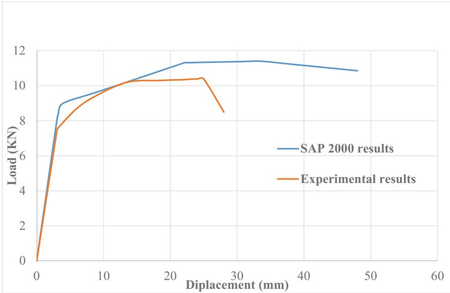
**Fig. 8.** Shows the static pushover curve generated from the SAP 2000 software and the formation of the first plastic hinge.
