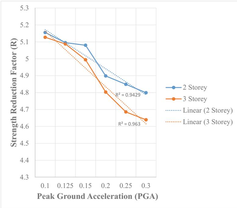
**Fig. 6.** Response modification factor R relationship with peak ground acceleration PGA.
