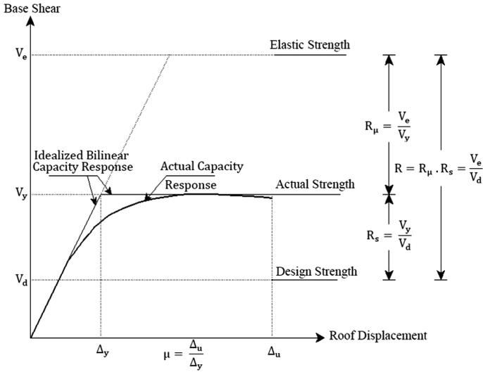
**Fig. 1.** Base shear  $V$  - Roof displacement  $\Delta$  relationship showing response modification factor  $R$  components ductility reduction factor  $R_\mu$  and overstrength factor  $R_s$ .
