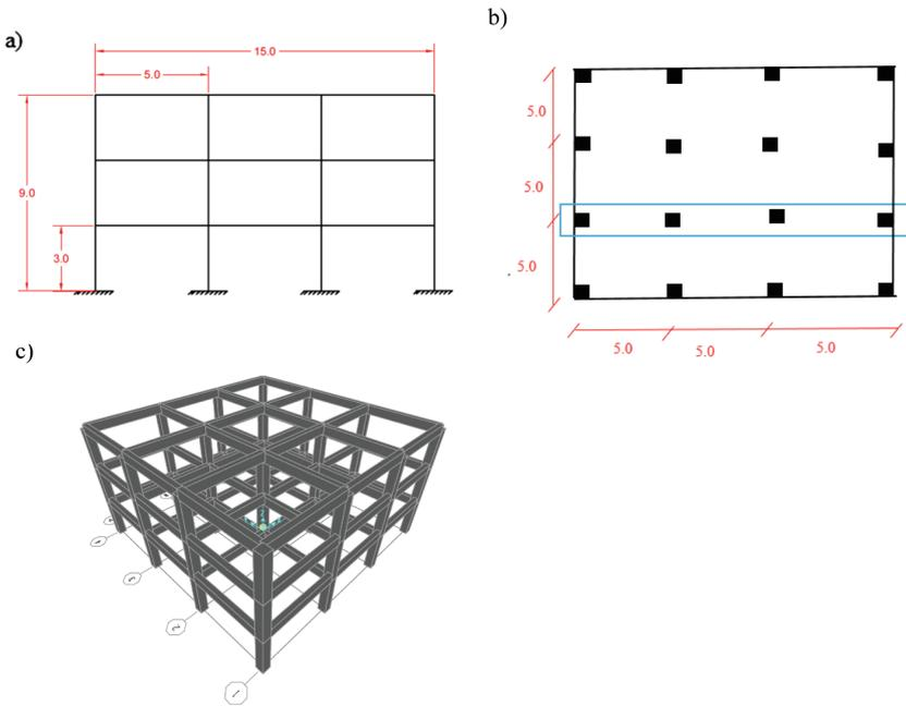
**Fig. 3.** For the 3 storey building (a) Elevation. (b) Plan. (c) Isometric view.
