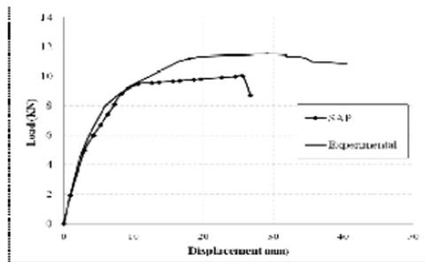
**Fig. 7.** Shows the BF model after pushover testing and its pushover curves
