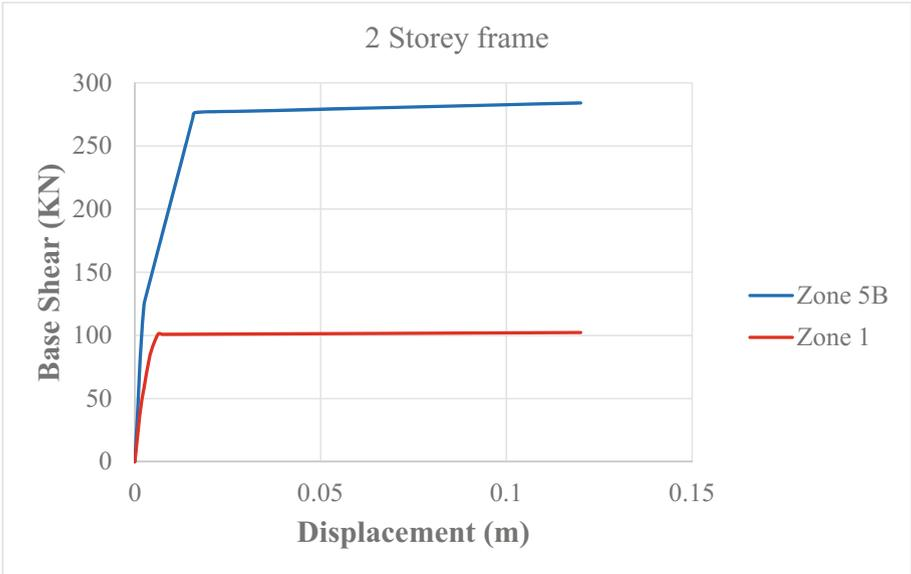
Fig. 4. Static pushover curve for 2 Storey frame in seismic zone 1 and zone 5B
