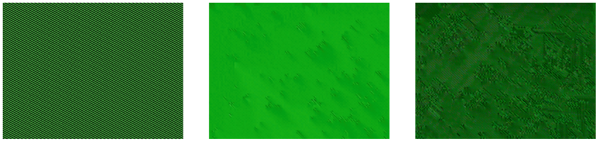
(a) Original pattern of the test case rotating around the center of the image. (b) Result frame showing grain like random artefacts. (c) Result frame showing randomly grouped artefacts.
