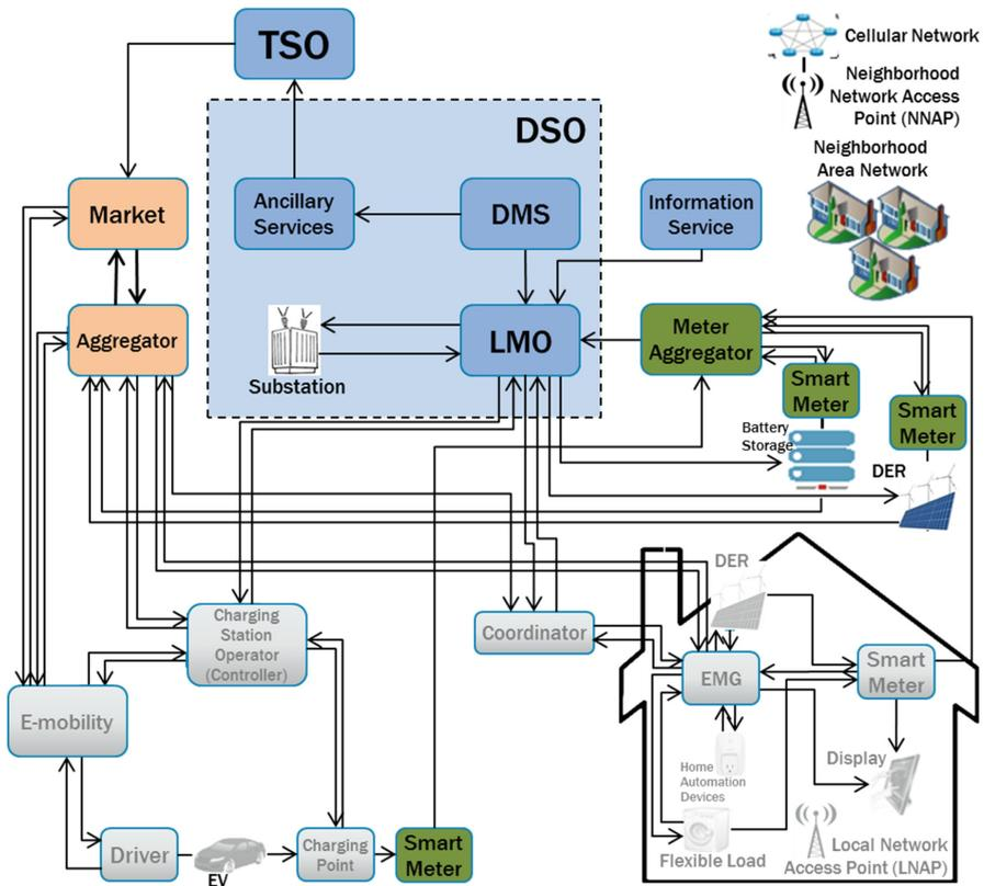
Fig. 22. Architectural view of Medium Voltage Control (3).
