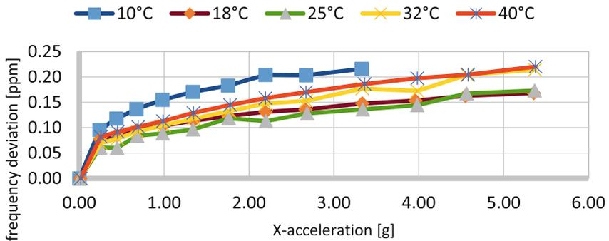
Fig. 5. Frequency deviation with respect to acceleration in X-axis at different temperatures.
