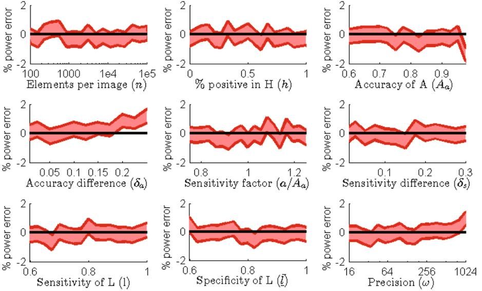
**Fig. 2.** Model accuracy: 95% confidence regions on the power prediction error (%). Values where the region does not contain the 0% error line suggest prediction error.
