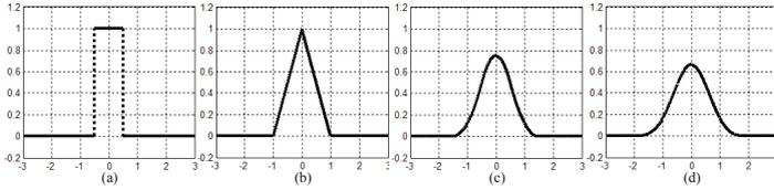
**Fig. 1.** One-dimensional B-splines with four different orders: (a)  $\beta^0(x)$ ; (b)  $\beta^1(x)$ ; (c)  $\beta^2(x)$ ; (d)  $\beta^3(x)$
