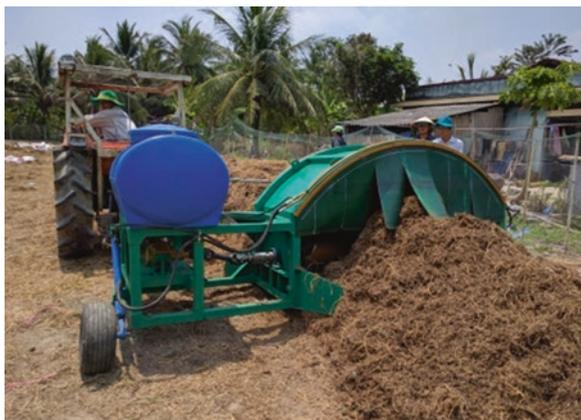
**Fig. 3.3b** Structure of the compost turner designed under the BMZ-IRRI project (IRRI 2019)
