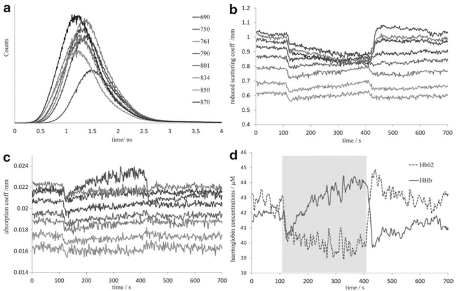
**Fig. 24.3** (a) Example TPSFs for single measurement. (b) Reduced coefficient of scattering for eight wavelengths over course of cuff occlusion. (c) Coefficient of absorption for eight wavelengths over course of cuff occlusion. (d) Concentration changes for HbO<sub>2</sub> and HHb, cuff inflation time of 4 s
