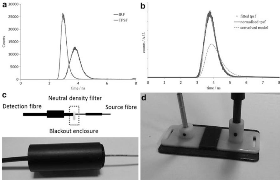
**Fig. 24.2** (a) Raw TPSF (scaled) and IRF, (b) theoretical model convolved with the IRF, the real TPSF and fitted curve using the lsqcurvefit function returning  $\mu_a$  and  $\mu_s'$  as 0.0224 and 1.0655  $\text{mm}^{-1}$ . (c) Method of measuring IRF. (d) 3D printed optode holder
