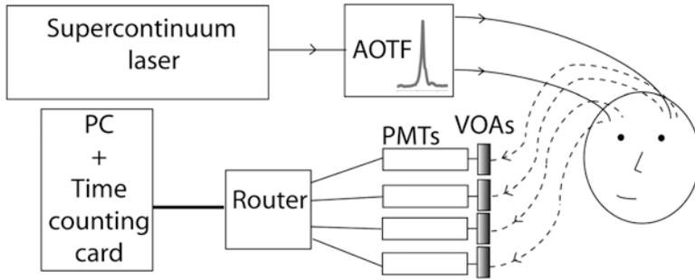
**Fig. 24.1** Schematic of time resolved multiwavelength near infrared spectrometer. The light is tuned using acousto-optic tunable filters (AOTF) and detected with four photomultiplier tubes (PMTs) each protected by variable optical attenuators (VOAs)
