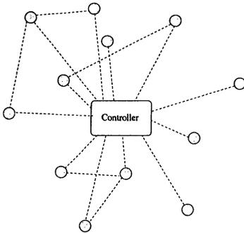
*Figure 3* Model 3. Mesh topology. Nodes can learn the centrally-mandated policy from other nodes as well as from the controller. Since the mesh topology does not assure direct connection to the controller, each node is responsible for its own policy enforcement.
