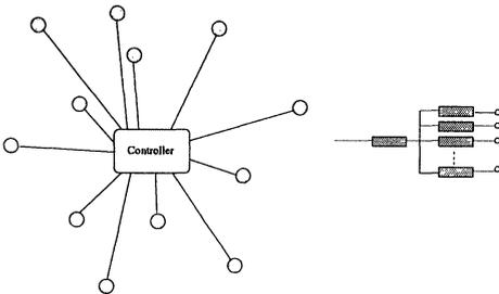
Figure 1 Model 1: the star network. A central manager maintains bi-directional communication with all clients. The links are perfectly reliable, and all enforcement responsibility lies with the central controller.
