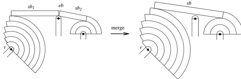
**Fig. 5.** A merge event. Vertex  $v$  pushes the left straight bundle  $sb_1$  up such that the elbow bundle  $eb$  in the middle disappears. The straight-elbow-straight bundle sequence  $sb_1 - eb - sb_2$  gets replaced by a single straight bundle  $sb$ .
