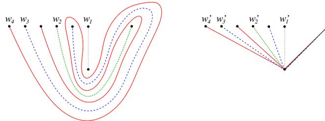
**Fig. 1.** An example with exponential complexity:  $k = \Omega(2^n)$ : On the left is the initial wiring sketch, and on the right is the wiring after the shortest paths have been computed. The number of edge segments in the shortest paths  $w'_1, w'_2, w'_3, w'_4$  is 1, 2, 4, 8. In general, wire  $w'_i$  has  $2^{i-1}$  edge segments. Note that on the right many edge segments are parallel.
