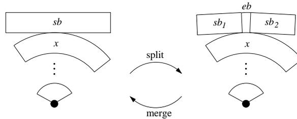
**Fig. 3.** Split and merge operations. The split operation splits the straight bundle at an elbow bundle into a straight-elbow-straight bundle sequence. The merge operation merges a sequence of straight-elbow-straight bundles into a single straight bundle.
