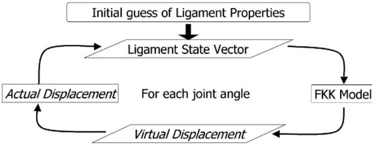
**Fig. 2.** The iterative process of UKF parameter estimation. When a new observation becomes available, the current estimate of the state vector is used to predict the femoro-tibial contact locations using the FKK model. The difference in the predicted and the observed femerotibial contact locations, call the *innovation*, is used to correct the state vector estimation.
