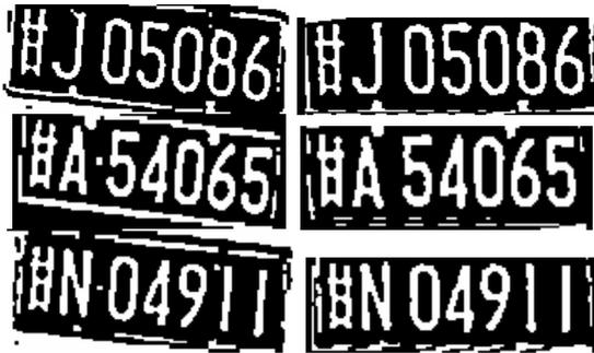
Fig. 10. Examples of horizontal slant corrections
