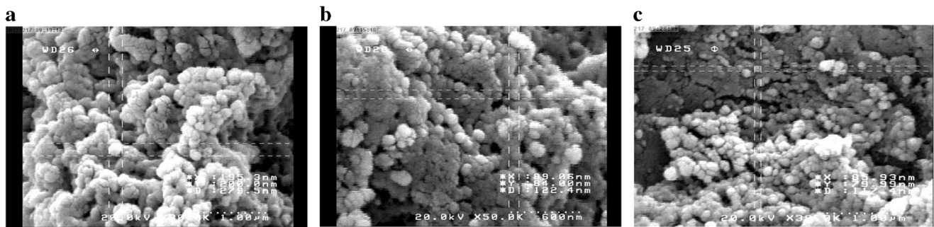
Fig. 5. SEM of non-MINP-32 (a, ×18,000), unwashed MINP-32 (b, ×33,000), and washed template (c, ×21,000)
