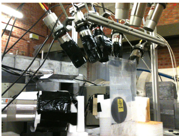
Fig. 6. (Color online) Photograph of GLADIS, the new Geel Lathanide halide Detector array for Isomer Studies presently consisting of 4 HPGe detectors (45% rel. eff.) and 8 cerium-bromide detectors of size 5.1\text{ cm} \times 5.1\text{ cm} (diameter \times length), taken during commissioning at a neutron flight-path station at JRC-IRMM.
