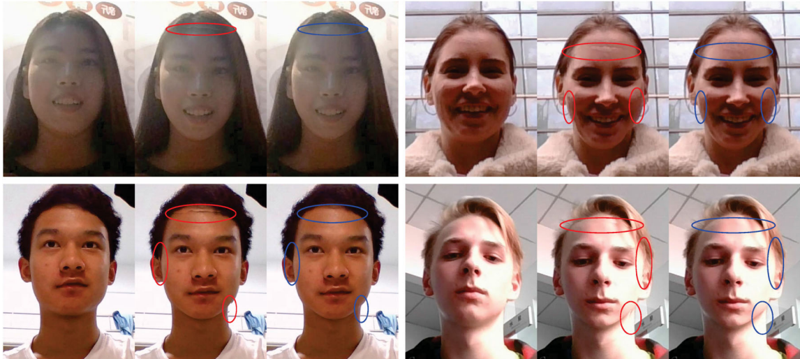
Fig. 6 Further examples of seam optimization and Laplacian blending. In each case, left to right: original image, corrected image after seam optimization, and final image after Laplacian blending. Red ellipses: visual artifacts. Blue ellipses: improvement after Laplacian blending.
