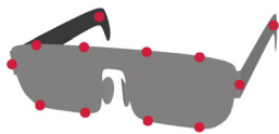
Fig. 7 Template mesh and the corresponding 12 landmarks (indicated with red circles) used in 3D glasses reconstruction.
