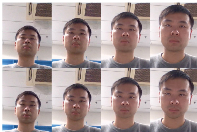
Fig. 13 Above: input frames for a user quickly approaching the camera. Below: correction results
