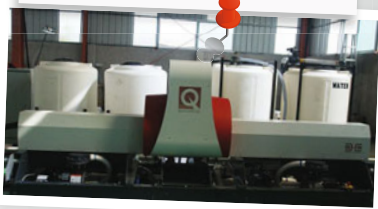
(Above) Quantum Design developed and installed its first superconducting high-gradient magnetic separator in China.
