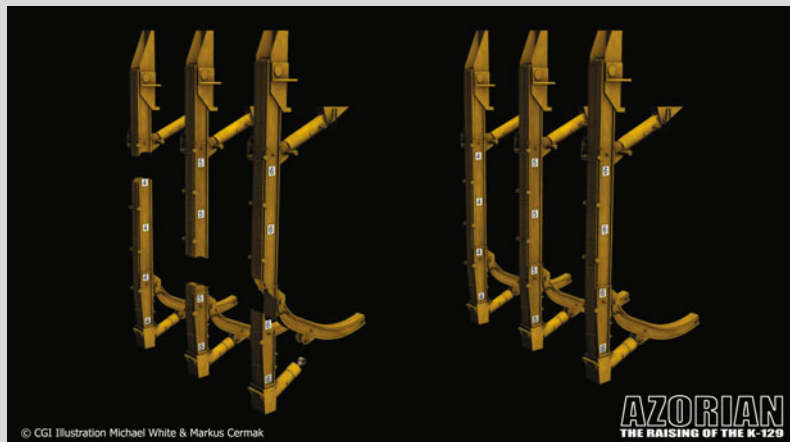
Figure 3. CGI illustration of the failed CV tines (left) and the CV tines prior to use. Note that the fractures occurred in different locations and the fractures do not appear brittle (i.e., straight). The fractures in all of the three fractured tines appear quite tortuous. Tine #4 failed on the ocean bottom and tines #5 and 6 failed during the final phase of the lift operation. Courtesy Michael White.
