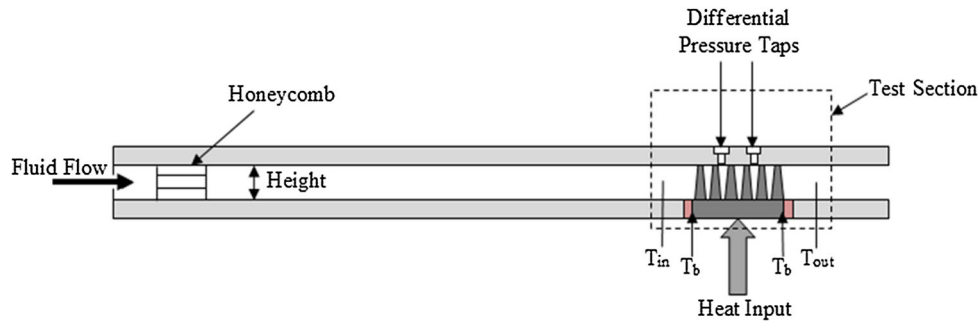
Fig. 5 Heat transfer fixture utilized to evaluate the fin arrays heat transfer performance
