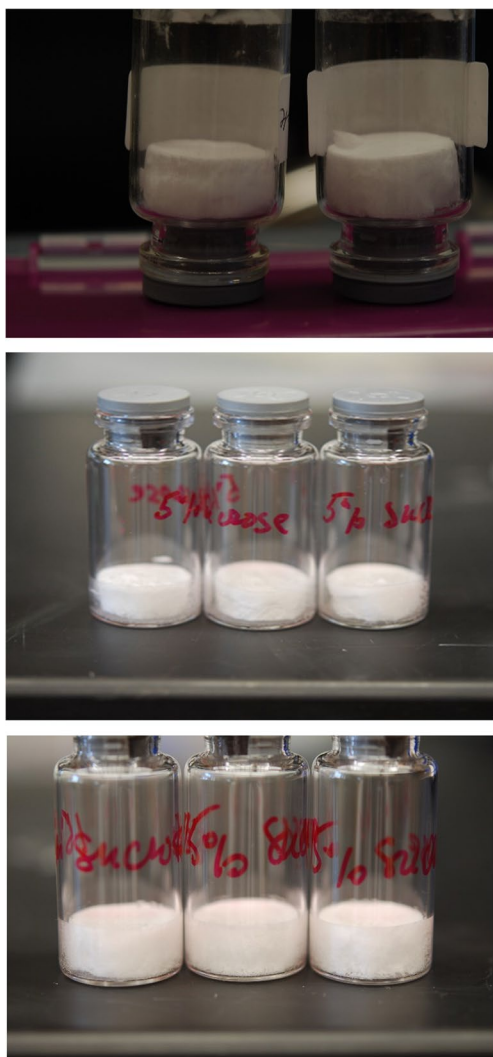
Fig. 11 Cake appearance of 5% (top picture, left vial) and 15% (top picture, right vial) of sucrose lyophilized below microscopic collapse temperature (shelf temperature of -28°C and pressure of 50 mTorr resulting in product temperature below -36°C and 33°C for 5% and 15% of sucrose respectively). Lyophilized cakes are shown upside down to demonstrate no collapse at the bottom of cake. Middle and bottom pictures are 5% and 15% sucrose formulations, respectively, lyophilized at or slightly above microscopic collapse temperature (-32°C for 5% and -30°C for 15%) using shelf temperature of -10°C and pressure of 100 mTorr.
