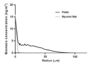
**Fig. 5** Biomass density profiles (kg biomass/m<sup>3</sup> of pellet volume) for the pellet and mycelial mat morphologies showing increased density at the pellet/mat core and the larger density of the pellet morphology
