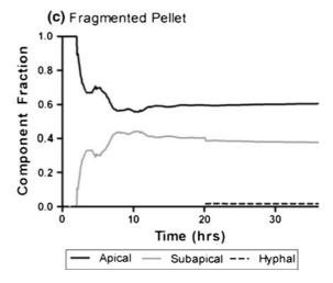
**Fig. 7** Comparison of component fractions (apical, subapical and hyphal) in simulated mycelial morphologies: **a** pellet, **b** mycelial mat, **c** fragmented pellet, plotted over time
