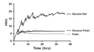
Fig. 6 HGU values for simulated dense pellet, mycelial mat and sheared pellet morphologies over time
